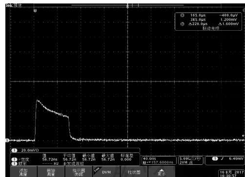
图6 锐科激光器波形图(58 ns,500 kHz) Fig.6 Waveform of Raycus laser(58 ns,500 kHz)
